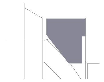
In the late 1960's the introduction of patented **Multi-Seal Technology** continued the advancement of seat design introducing auxiliary blunt edged sealing faces that provided 1 low pressure and up to 2 high pressure sealing contacts. The blunt edged auxiliary faces allowed for grooves to collect and trap particulates for removal over multiple open and close cycles.
