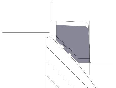
"Operational and Environmental demands challenging the Energy Industry are driving the need for an improved floating ball valve seat design that provides progressive sealing surfaces in both low and high pressure applications"
