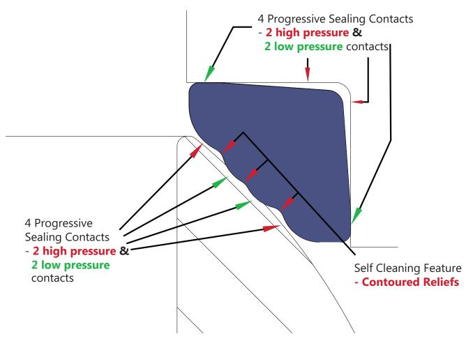
EDi's **Progressive Seal Technology™\*** introduces 4 Contoured Front Sealing Faces and 4 Flat Backside Sealing Faces that dramatically improve low and high pressure bubble tight sealing in floating ball valve applications. The dynamically energized seat is designed to be self relieving on the upstream side reducing operating torques.
